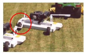
The rear hitch (Part # 900009 used on Models H40B, H60B & C60BE or Part # 900137 used on Models Pro60K) is used for hitching two AcrEase in tandem (both off to the left side).
