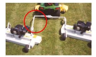
The long tongue extension (Part # 900008 used on Models H40B, H60B & C60BE or Part # 900136 used on Models Pro60K) is used when two AcrEase are pulled (one on the left and one on the right). By extending the left side AcrEase back, grass will not be blown onto the right side AcrEase.
