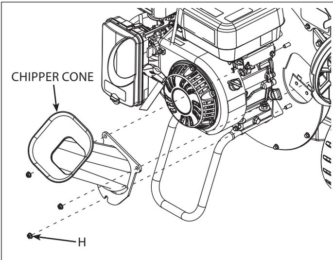
Position the chipper cone over the three M8 x1.25 threaded studs protruding from the engine plate, and attach using three M8 nyloc nuts (H). Rotate cone and cone base away from engine so cone does not contact engine. Tighten the three M8 nyloc nuts (H) securely.
