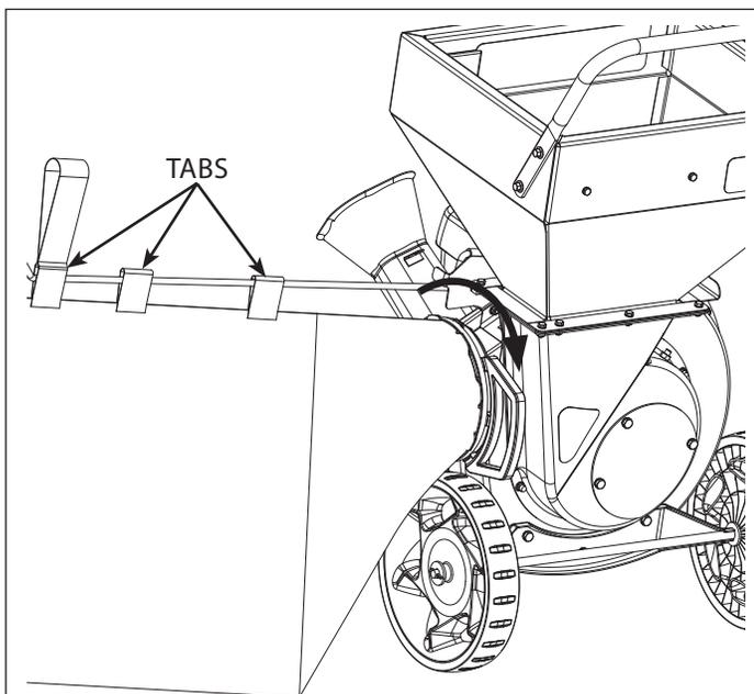
Slide the tabs on the debris bag onto the support rod. Secure the bag connector onto the chipper by rotating the connector until locked in.
