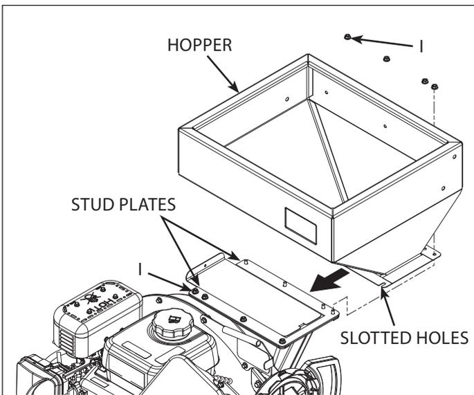
Install hopper by sliding slotted holes on the front side of hopper onto the four studs on the front stud plate with the previously loosened four M6 nuts (I). Reinstall rear stud plate and back four M6 nuts (I) that were previously removed in Figure 4. Tighten all eight M6 nuts (I).
