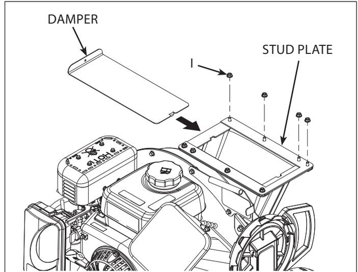
Remove back four M6 nuts (I) and set nuts and rear stud plate aside. Loosen front four M6 nuts (I). **Note: These will not need to be removed.** Install the damper between the stud plates as shown.
