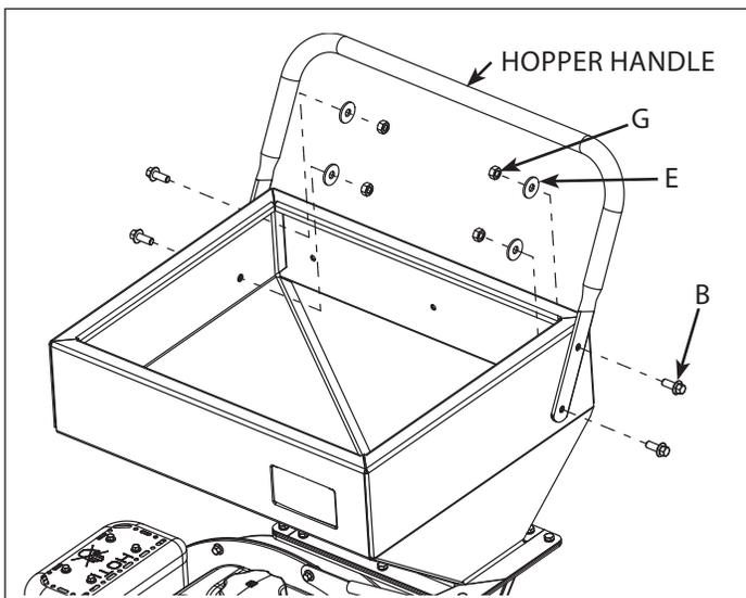
Hold the hopper handle up so that the outer holes in the handle align with the holes in the hopper and secure with four M8 x 20 MM bolts (B), four M8 washers (E) and four M8 nuts (G). Insert the screws from the outside of the hopper.
