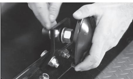
**STEP 4:** Install the skid shoe bracket cupping upwards.
