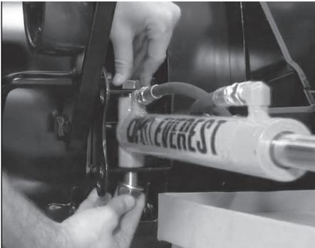
**STEP 15:** Hook large springs onto the top of the blade assembly.
