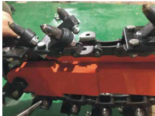
STEP 4: INSTALL CHAIN PLATE WITH PINS
