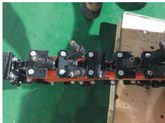
STEP 6: TIGHTEN ALL BOLTS
