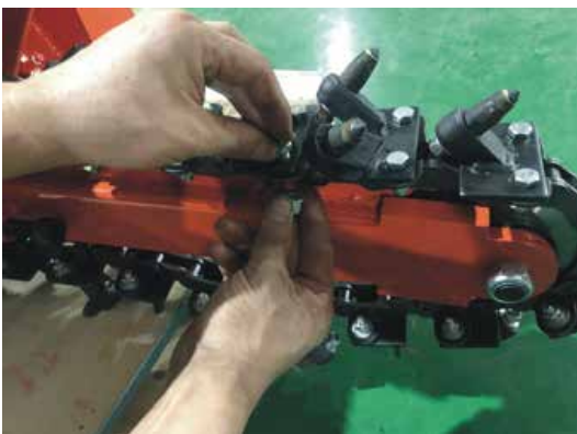
STEP 5: FINISH BLADE HOLDER INSTALL
