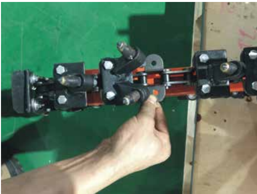
STEP 3: INSTALL CHAIN PLATE JOINT
