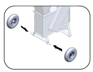
2. Insert 5/8" flat washer before inserting safety cotter pin as shown on figure below. Twist the ends of the cotter pin with some pliers to avoid losing the pins.
