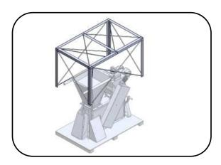
**4.** Remove the chipper by unscrewing the shipping fasteners. See figure below.
