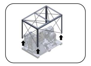
**4.** Remove the grinder removing the platform anchoring ships. See Fig.
