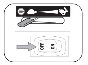
**2.** Shut the fuel valve and turn the engine switch OFF.
