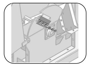
**NOTE:** To remove the blade's bolts, it is recommended to place a piece of wood in between the rotor and the outside edge to
