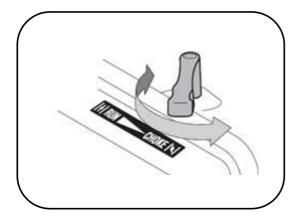
3.Move the lever throttle control to the fast position.See the figure.
