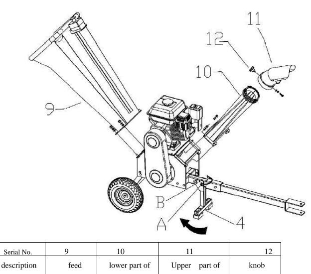
1.Connect the hinger of lower part of outlet hopper10 to the one on the frame with screw nut, then put the upper part11 on the lower part10 with bolts and knob12.
